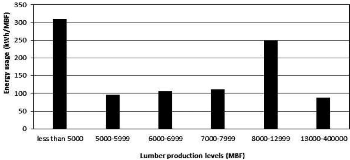
Figure 3.—Energy use per thousand board feet (MBF) of lumber production by production levels.
