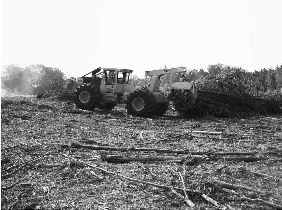
Figure 5.—Tigercat 630D with 635 grapple skidding timber.
