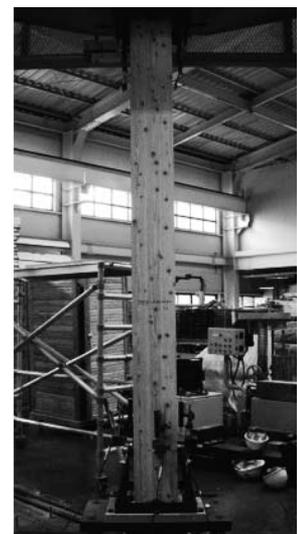
Figure 4.—Axial compression test method.
