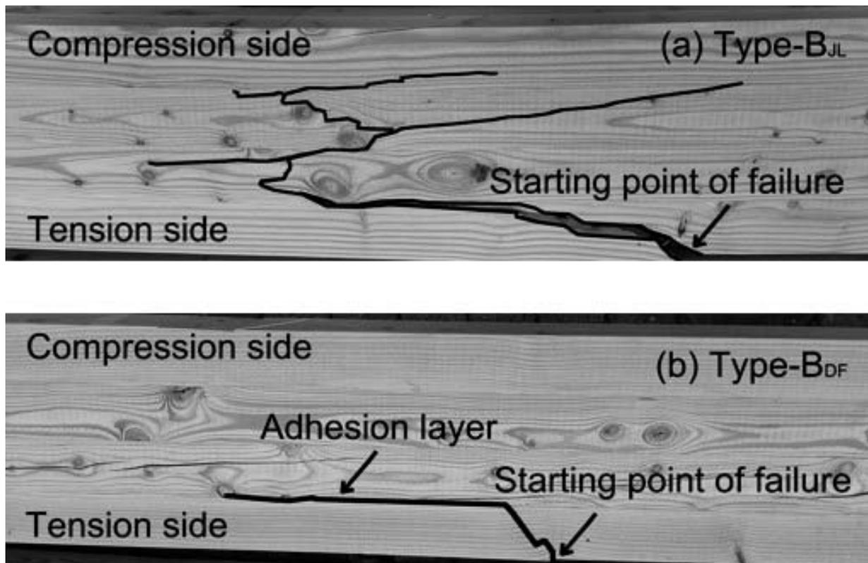
Figure 6.—Bending failure mode for laminated beams.
