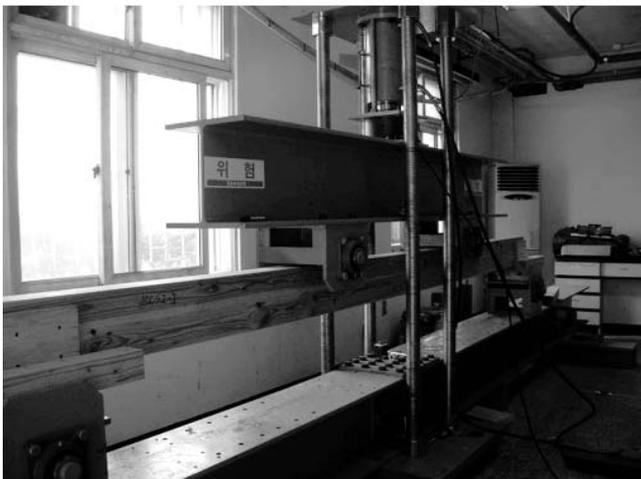
Figure 3.—Bending test method.
