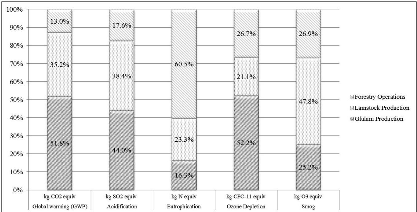
Figure 3.—Contribution analysis life-cycle impact assessment per 1 m<sup>3</sup> of glued-laminated (glulam) timber production in the Southeast (mass allocation).
