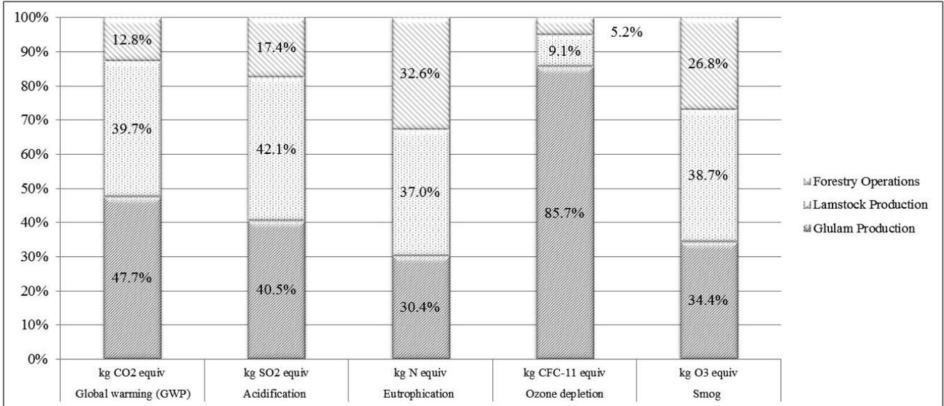
Figure 2.—Contribution analysis life-cycle impact assessment per 1 m<sup>3</sup> of glued-laminated (glulam) timber production in the Pacific Northwest (mass allocation).
