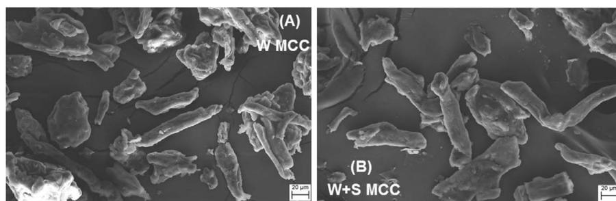
Figure 2.—Scanning electron microscopy images of (A) wax (W)-coated microcrystalline cellulose (MCC) and (B) wax and surfactant (WS)-coated MCC.
