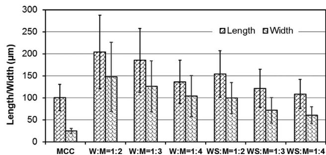
Figure 3.—Changes of lengths and widths of microcrystalline cellulose (MCC) particles before and after coating with wax (W) and wax and surfactant (WS).
