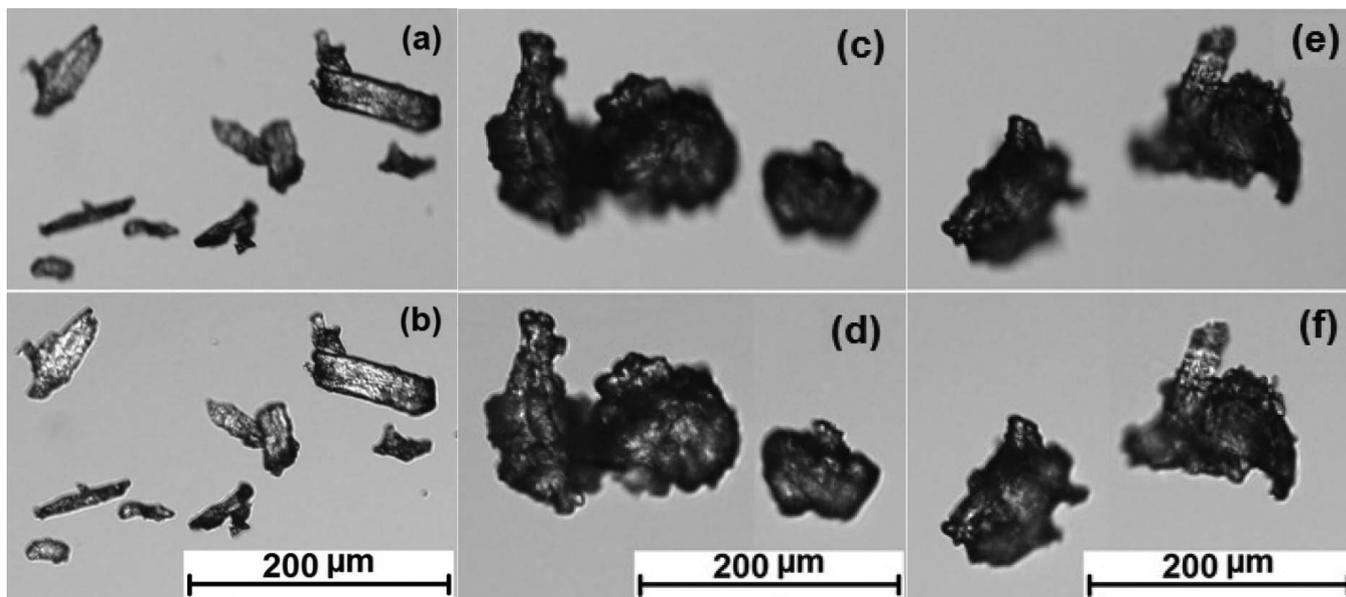
Figure 1.—Images of uncoated microcrystalline cellulose (MCC) (a, b), wax-coated MCC (c, d), and wax and surfactant-coated MCC (e, f) from regular light microscopy (a, c, and e) and differential interference contrast light microscopy (b, d, and f).
