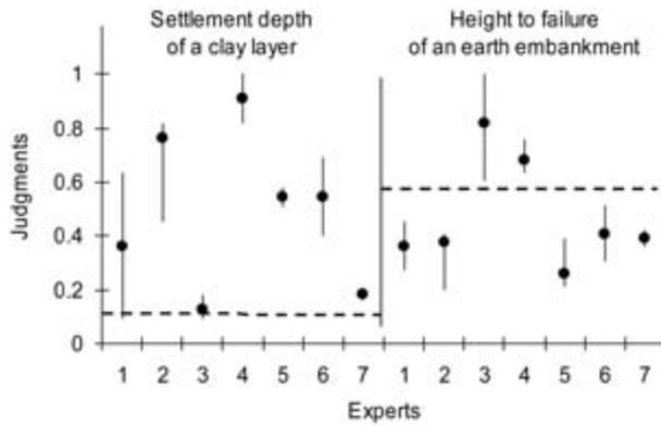
**Figure 3.** Opinions of geotechnical experts on two standard problems. The correct (measured) values for settlement depth was 1.5 cm and for added height to failure was 4.9 m. The x-axis for both was rescaled so the maximum value was 1. Correct values are shown as dashed horizontal lines. The intervals show 'minimum' and 'maximum' values reported by the experts (after Hynes and Vanmarcke 1975 in Krinitzsky 1993).
