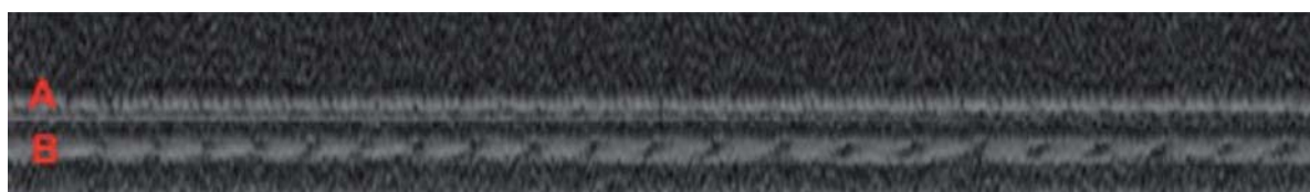
Figure 7. A is an insect wingbeat signature. B is a bird wingbeat signature Source: DeTect 2007
