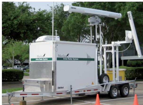
Figure 4. Horizontal and vertical antenna system Source: DeTect 2007
