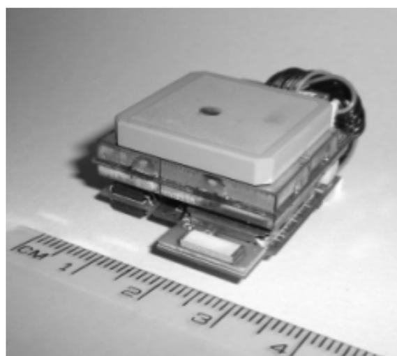
**Figure 2:** Assembled GPS unit – the small projection is the Bluetooth antenna.
