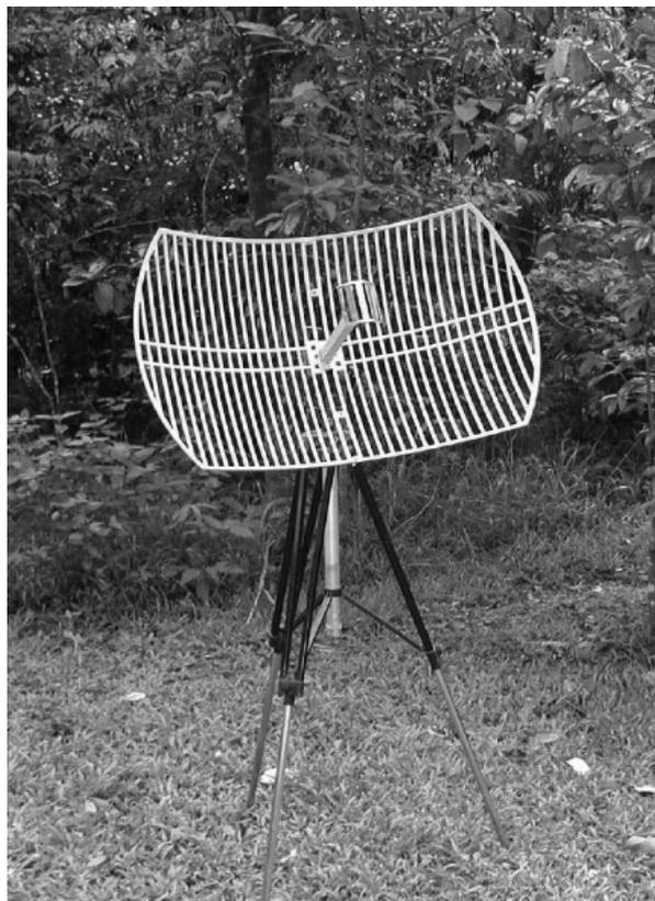
**Fig. 6:** This 2.4 GHz, 26dB gain antenna is capable of ranges of about 250 m in open forest (assuming you can detect the beacon transmission of course!!).
