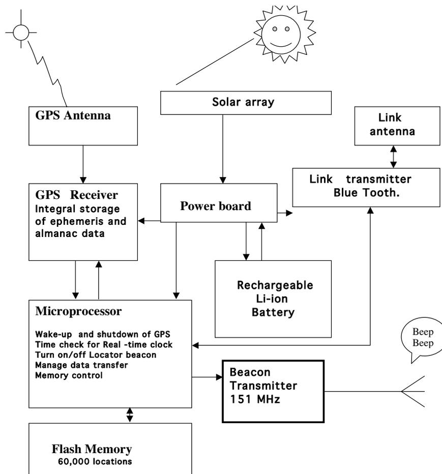
Figure 3: Block schematic of the GPS logger.
