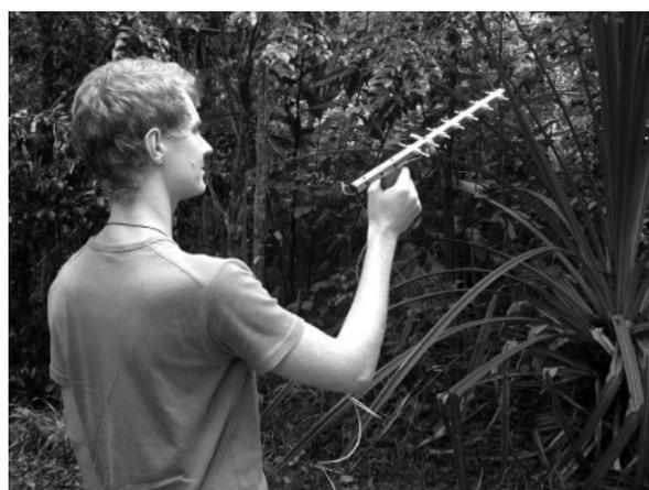
**Fig 5:** A handheld 2.4 GHz antenna like this (8db gain) is adequate for downloading data over a distance of one hundred metres. It would be 'piggy-backed' on a conventional 151 MHz radio-tracking array (used to find the beacon transmission).
