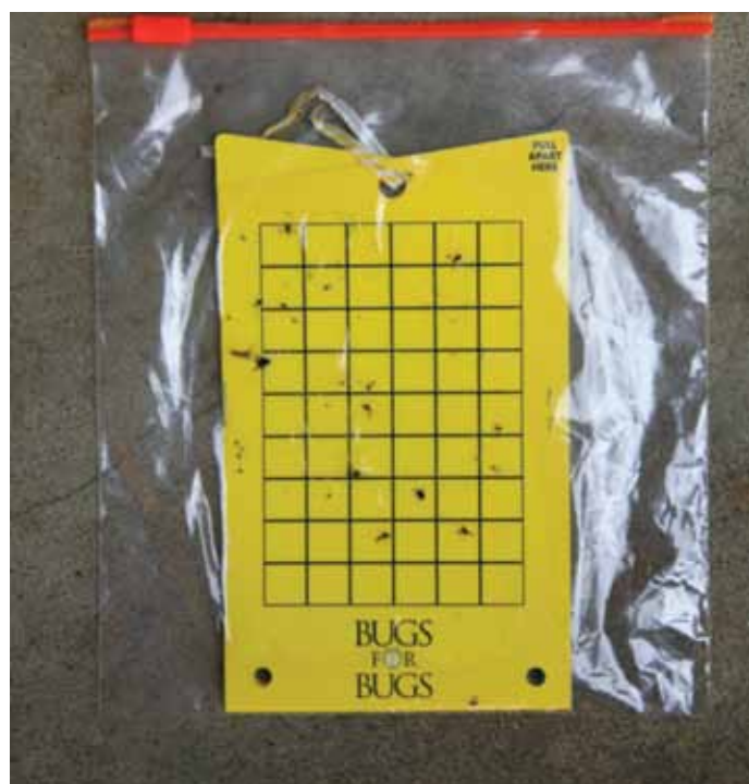
Figure 5. Yellow sticky trap showing grid, placement in plastic zip lock bag, and an example of the catch (since this was a 'prototype' there is no hole at the centre right for orientation.) Photo, M. Dingley.
