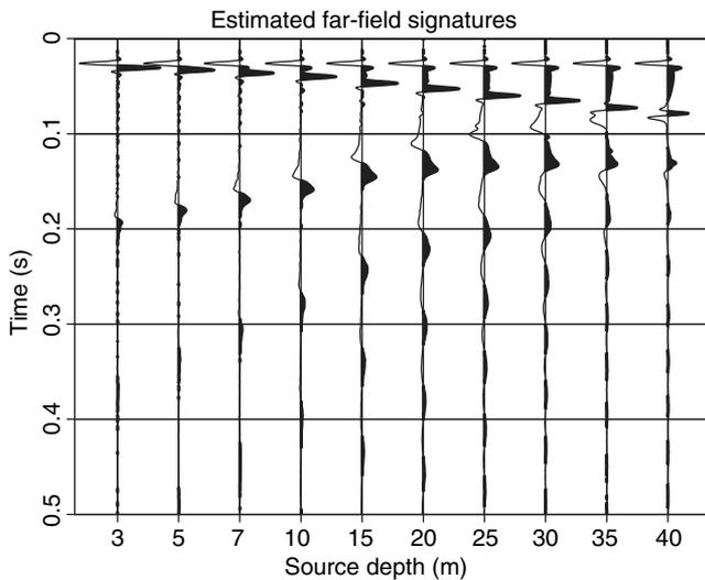
Figure 1. The estimated far-field signatures for zero offset from a single 600 in<sup>3</sup> air gun fired at depths ranging from 3 to 40 m. Note how the bubble pulse delay is reduced as the source depth increases. Also note the free-surface ghost and how it is delayed as the source depth increases.
