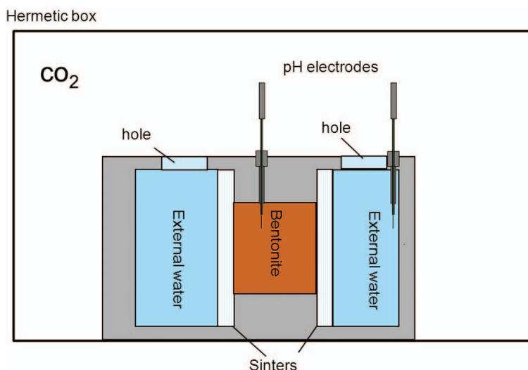
FIG. 1. Schematic picture from the experimental setup.
