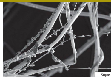
A spider's web heavily loaded with particulate matter from a car transportation site in Wrocław city.
