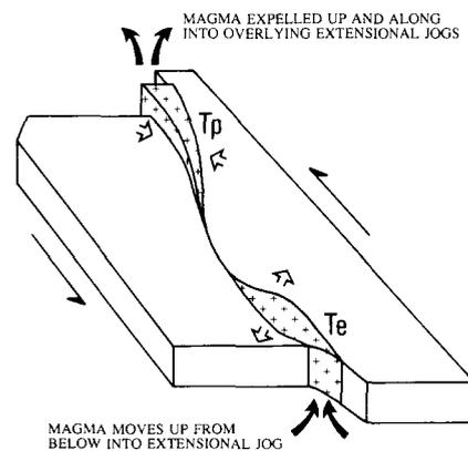
**Fig. 2** Cartoon depicting a general mechanism for the upward transport of magma within an evolving sigmoidal, strike-slip shear zone or fault, showing movement of magma (black arrows) into a zone of transtension (Te) and from a zone of transpression (Tp).
