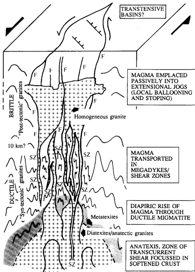
Fig. 3 Generalized model for the generation, ascent and emplacement of granite magma within mid- to upper crustal levels of a transpressional orogen (SZ, shear zone; F, fault).
