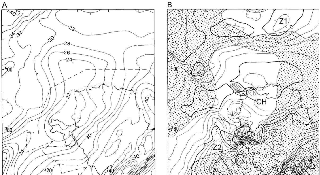
**Fig. 2.** (A) Bouguer gravity anomaly map of Anglesey and the adjoining areas. Contours at intervals of 2 mGal. Offshore contours from a recent BGS compilation of gravity data. Broken line indicates inshore limit of marine surveys. (B) Aeromagnetic anomaly map with contours at 20 nT intervals. The stippled areas have gravity values greater than 28 mGal. CH, Carmel Head thrust; Z1 and Z2 are referred to in text.
