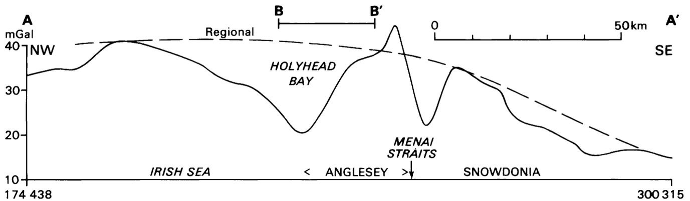
Fig. 3. Observed Bouguer gravity profile AA' across North Wales and part of the Irish Sea (see Fig. 1 for location). BB' is the projection of the profile shown in Fig. 4.
