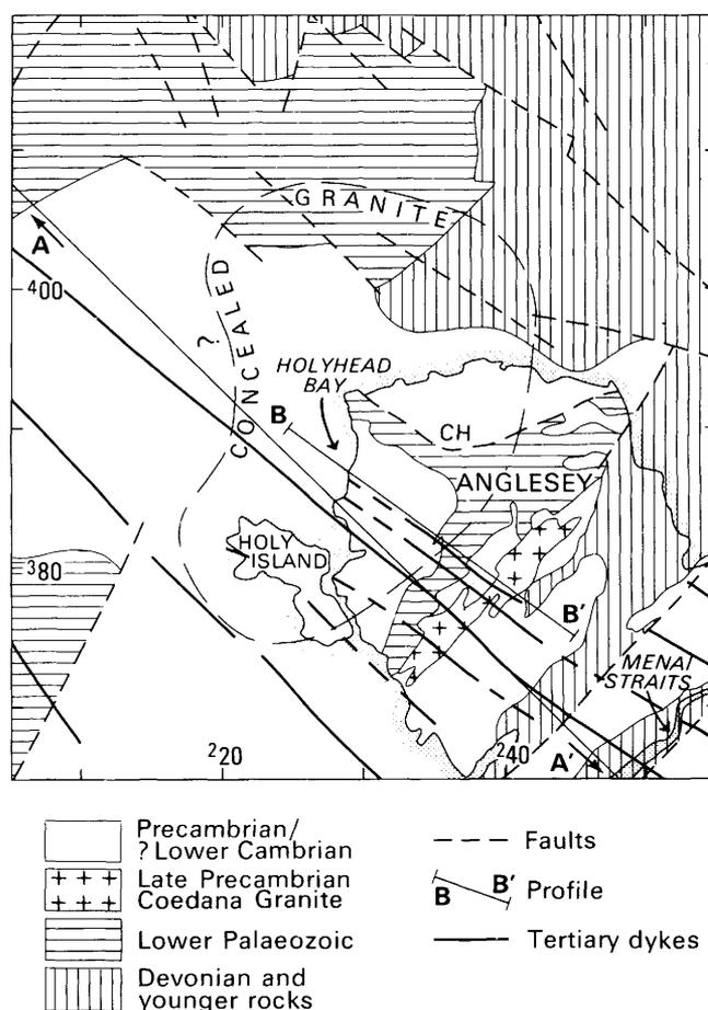
**Fig. 1.** Simplified geological map of Anglesey and adjoining areas with locations, based on geophysical evidence, of the postulated granite and Tertiary dykes. AA' and BB' are locations of profiles. CH, Carmel Head thrust. Ticks indicating the National Grid at 10 km intervals are shown at the margins of the map.
