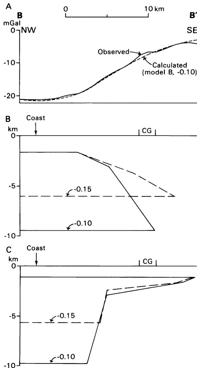
**Fig. 4.** (A) Residual Bouguer gravity data for the profile BB' (see Fig. 1 for location). The models shown (B and C) (with density contrasts in  $\text{Mg m}^{-3}$ ) are considered to be symmetrical about the coast and to have strike extents of 40 km. The calculated profile for one model only is shown; the others are very similar. Background gravity field +40 mGal. CG, Coedana Granite.
