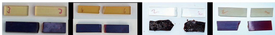
FIG. 1. Photographs of some of the candidate encapsulants before (top) and after irradiation to 10 MGy (bottom). From left to right: APS, Alchemix, Huntsman and VES.
