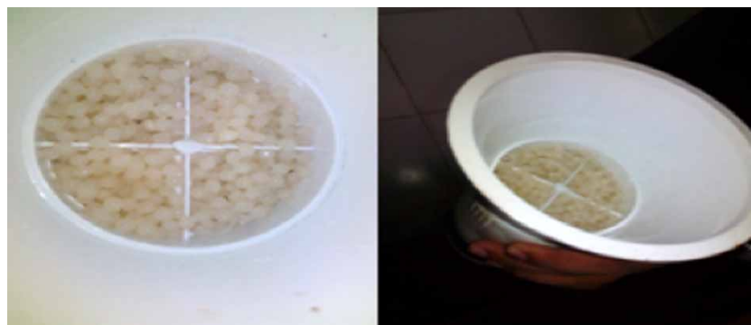
Figure 2 | Immobilised Ca-alginate beads inside the bioreactor system.
