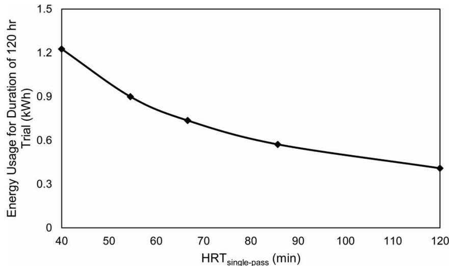
**Figure 6** | Relationship between HRT<sub>single-pass</sub> and energy usage for pumping.
