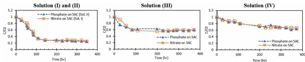
**Figure 4** |  $C/C_0$  versus time for solutions I-IV, showing increasing times for removal and decreased removals as solution complexity increases.
