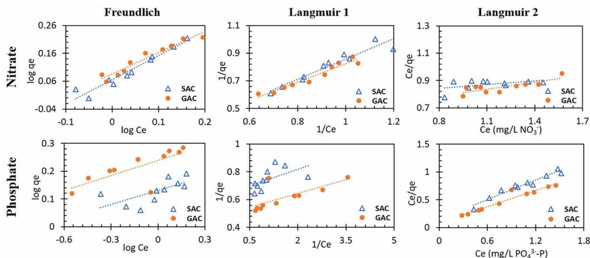
**Figure 2** | Adsorption isotherm models and adsorption capacity  $K$  (Freundlich) and  $Q$  (Langmuir) of SAC and GAC in solutions (I) and (II), respectively.
