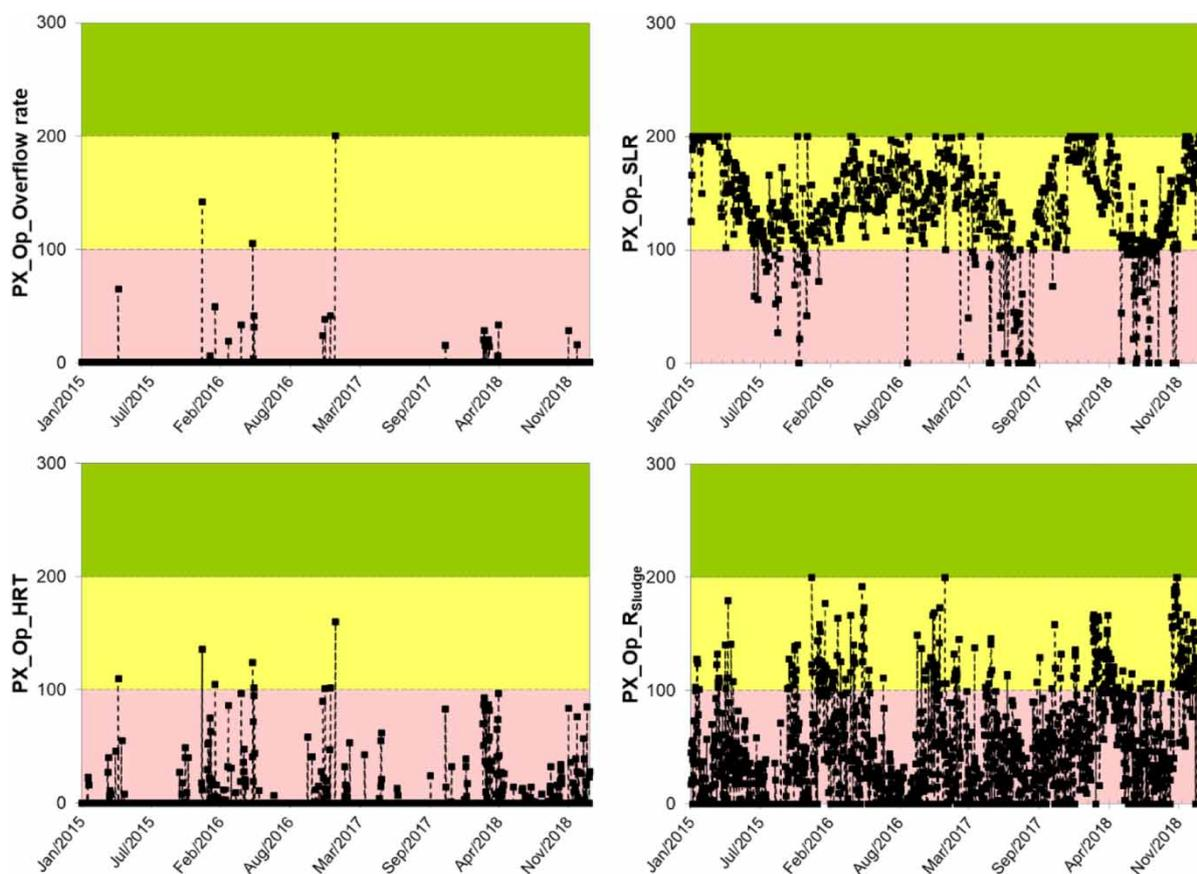
**Figure 5** | Performance indices for the secondary clarifier unit.
