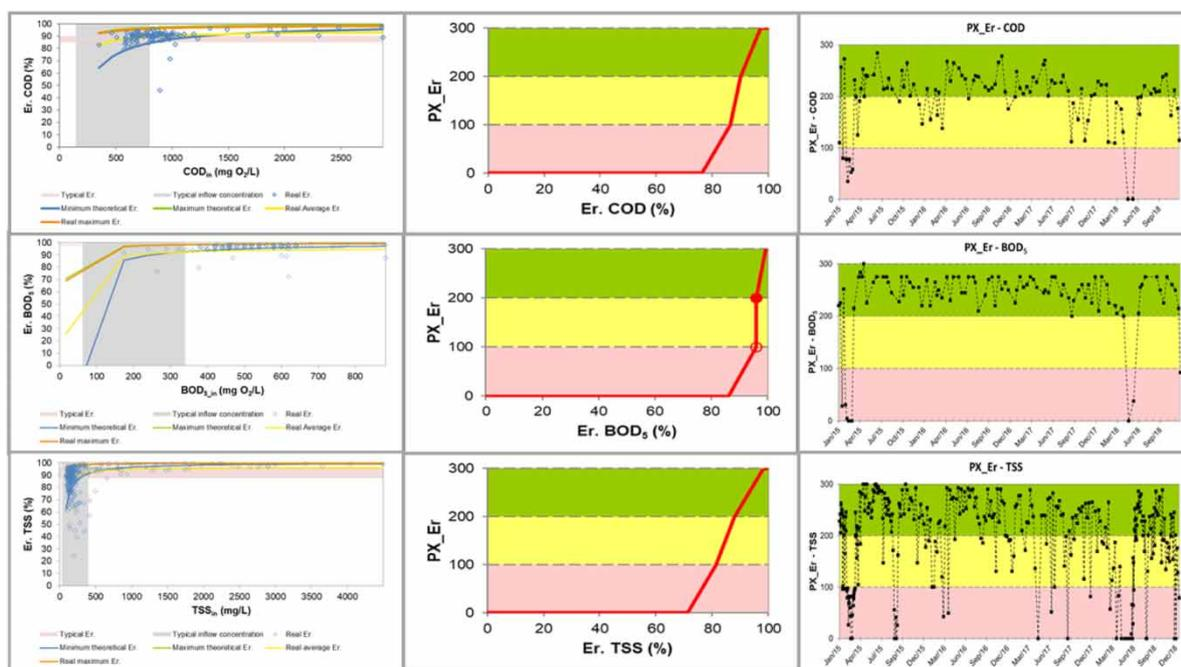
**Figure 4** | Er model curves (for theoretical and real Er), effect of  $C_{in}$  on Er and typical  $C_{in}$  range (left), examples of performance functions used converting removal efficiencies of COD, BOD<sub>5</sub> and TSS into PX\_Er (middle) and PX\_Er obtained for the studied WWTP (right).
