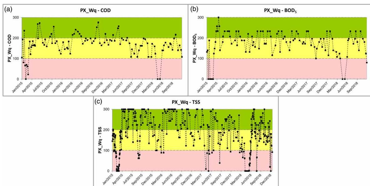
**Figure 3** | Daily performance indices of treated wastewater quality for COD, BOD<sub>5</sub> and TSS.
