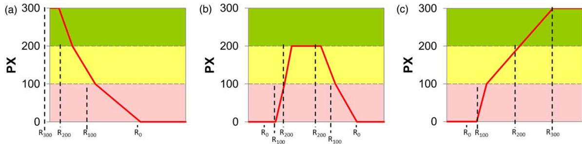
**Figure 1** | Performance functions used converting state variables of relevant operational performance assessment aspects of the WWTP into dimensionless performance indices. ( $R_0$  to  $R_{300}$  are reference values) (red – poor performance, yellow – acceptable performance, green – good performance).
