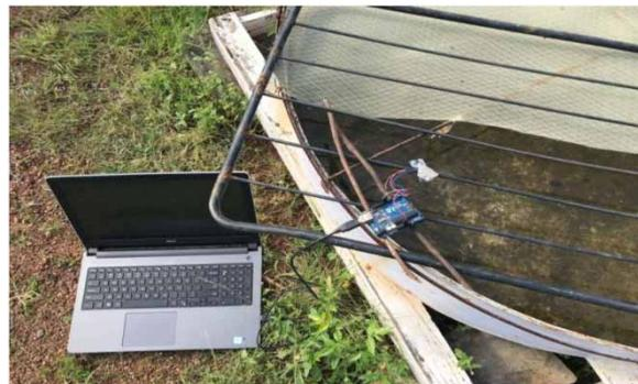
**Figure 4** | Sensors' calibration using evaporation pan.
