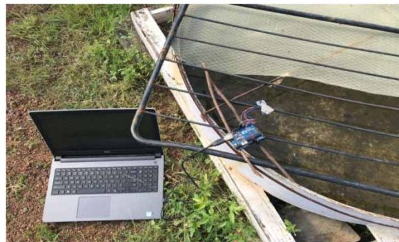
Figure 4 | Sensors' calibration using evaporation pan.
