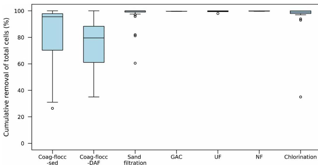
**Figure 2** | Cumulative removal of total cyanobacterial cells during treatment ( $n = 50$ ). Boxplots show the minimum, maximum, median, first quartile, and third quartile, and the circles reflect statistical outliers.
