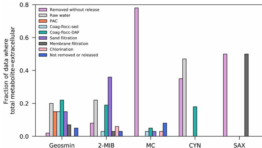
**Figure 5** | Stage of treatment where the concentration of extracellular metabolite was equal to the total metabolite concentration as a fraction of the total sampling events for geosmin, 2-MIB, MC (microcystin), CYN (cylindrospermopsin), and SAX (saxitoxin).
