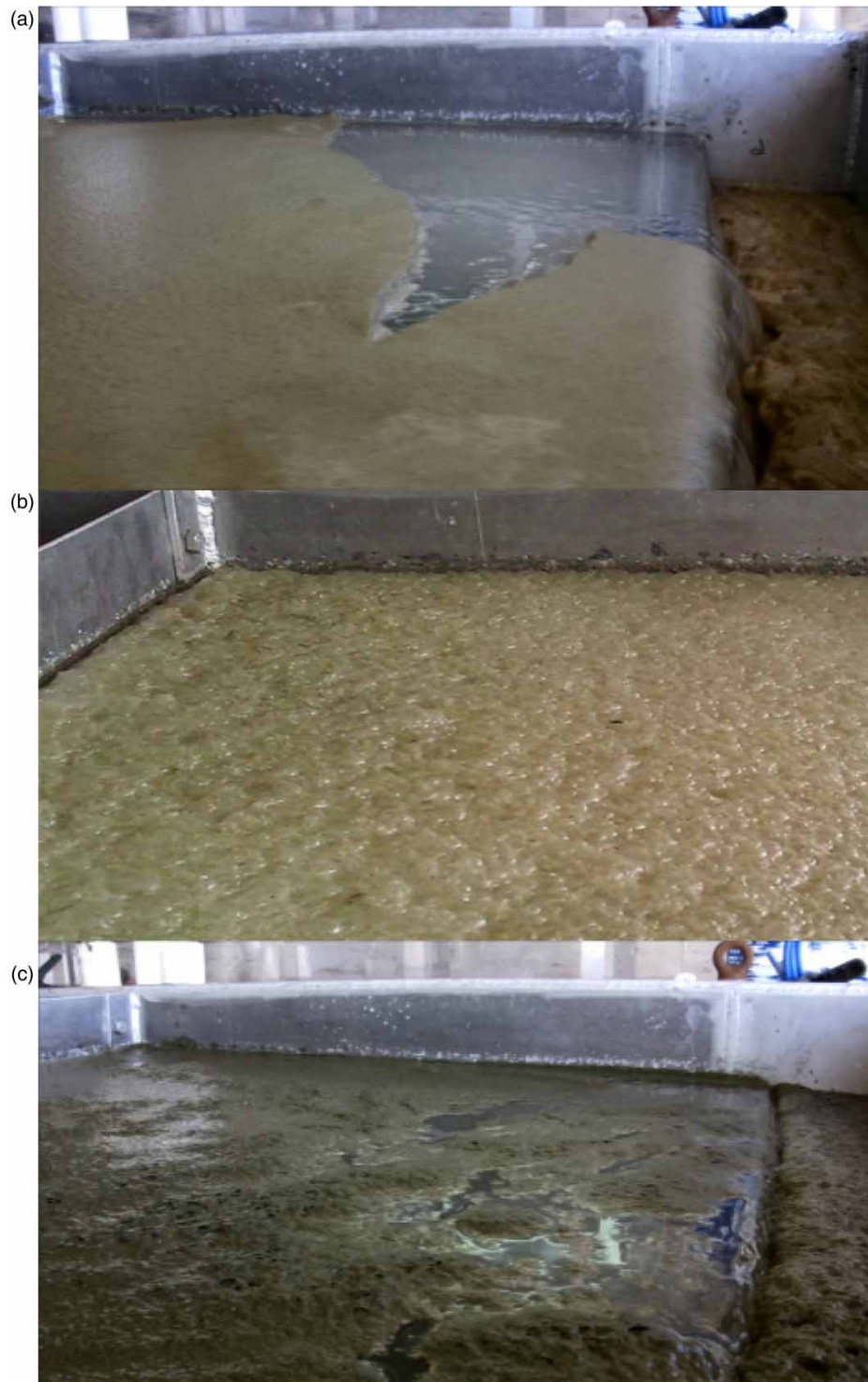
Figure 5 | Images of the float layer produced using (a) PosiDAF with PDADMAC, (b) PosiDAF with the HMP, and (c) conventional DAF. In PosiDAF, the float is removed as a sheet, whereas in conventional DAF, the float was observed to break up due to the shear forces during hydraulic removal.
