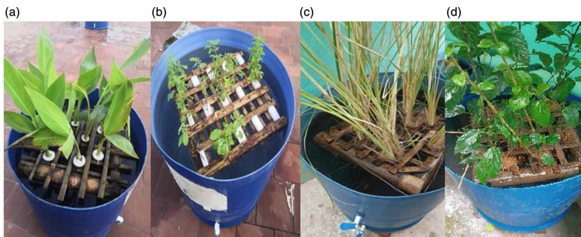
Figure 3 | FWT using (a) Canna indica , (b) Holy basil, (c) Vetiver, and (d) Hibiscus.
