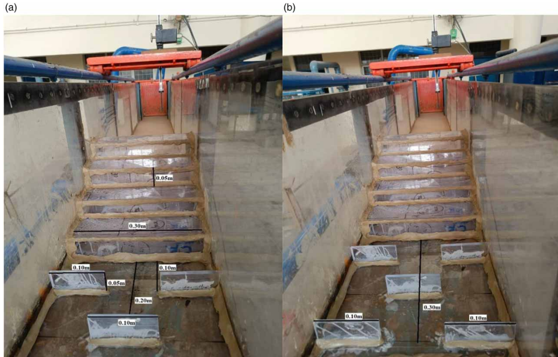
Figure 5 | Stepped spillway model with (a) three baffle and (b) five baffle configurations.
