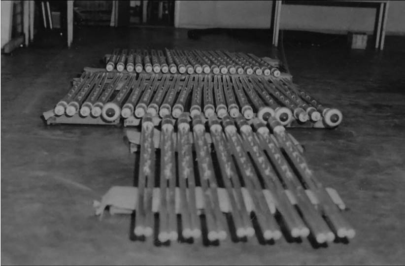
**FIGURE 5.** British uranium metal fuel rods, welded in pairs to fit the Norwegian reactor design. *Source:* Author picture from IFE, Kjeller, Norway.
