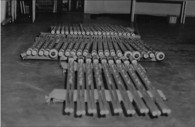
FIGURE 5. British uranium metal fuel rods, welded in pairs to fit the Norwegian reactor design. Source: Author picture from IFE, Kjeller, Norway.
