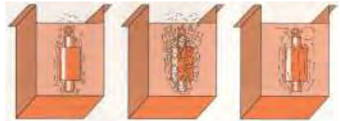
Figure 1 - Schematic showing the three phases of quenching. From left to right: Vapor Phase; Boiling Phase; and Convection Phase
