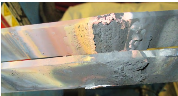
Figure 2: Example of copper and soot-like acetylene by-product build up on power feedthroughs
