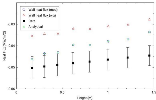
**Fig. 4** Heat flux for Kuhn test 3.5-2, which used air as a noncondensable
