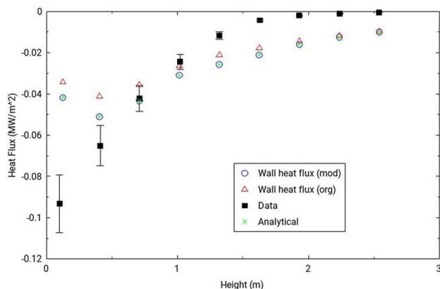
**Fig. 8 Heat flux for MIT test 18H, which used helium as a noncondensable**
