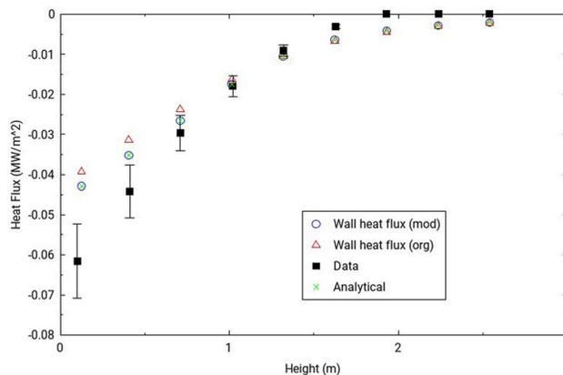
**Fig. 7** Heat flux for MIT test 8A, which used air as a noncondensable
