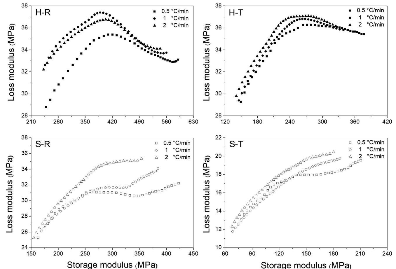
Figure 3.—Cole-Cole plot in heartwood and sapwood specimens in the radial and tangential directions at different heating rates. H-R = heartwood specimen in the radial direction; H-T = heartwood specimen in the tangential direction; S-R = sapwood specimen in the radial direction; S-T = sapwood specimen in the tangential direction.
