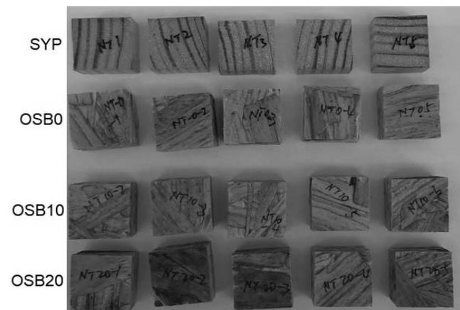
Figure 6.—No-termite control samples after 4 weeks on moist sand and oven-drying.
