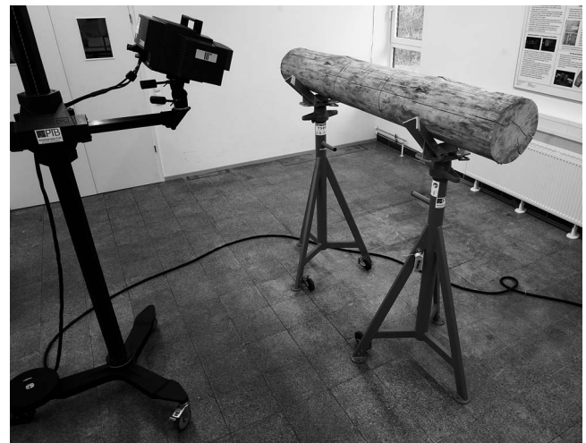
Figure 1.—Log (length 2 m, diameter 280 mm) on two supports in Bessel configuration before the start of fringe projection scanning. The scanning head of the fringe projection system containing the pattern projector and the cameras is seen on the left.
