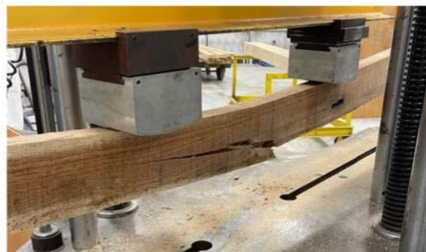
Figure 2.—Red oak lumber on Tinius Olsen machine before (upper panel) and after failure (lower panel) with the type of failure in static bending cross-grain tension (ASTM D143-14 [ASTM 2017a]).
