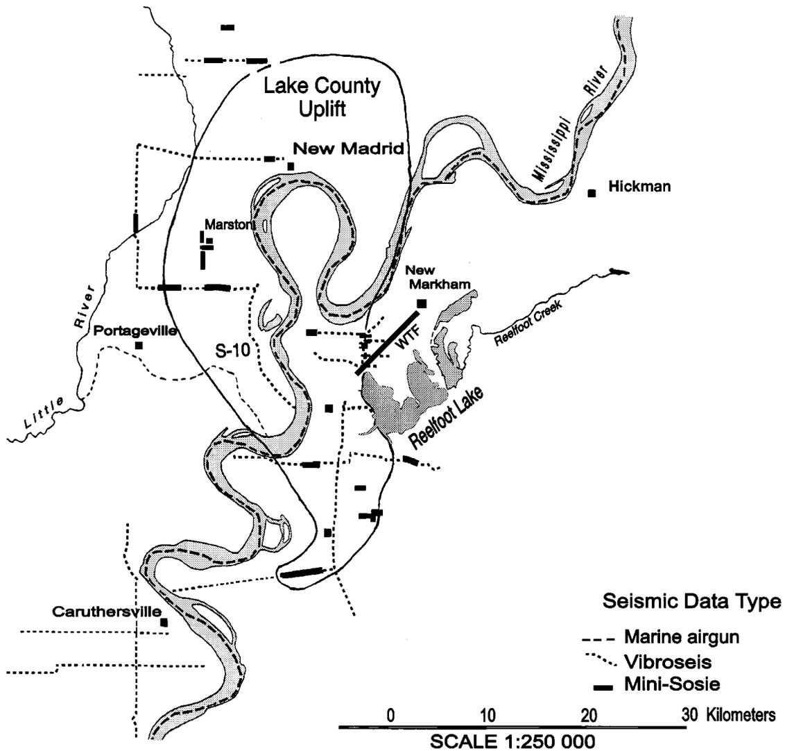
Figure 2. Location map showing the distribution and type (air gun, Mini-Sosie, and Vibroseis) of seismic reflection surveys in the New Madrid seismic zone. Base map is modified from Rhea and Wheeler (1994).
