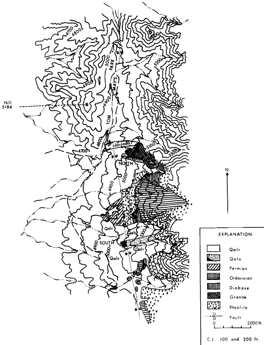
Figure 2. Geologic map of North Franklin Mountain remnants of early to middle Pleistocene piedmont deposits. The geology shown on this map is that pertinent to the problem only. The Jornada surface is shown locally north of the north remnant of older alluvium (Qalo). Qalr is shown only at a few important localities.
