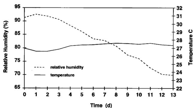
Fig. 1. Relative humidity and temperature conditions in a controlled environment used for slow curing of peanuts.
