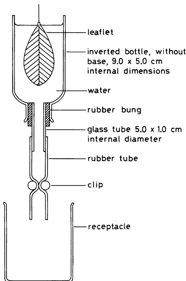
Fig. 1. Diagram of the constant drainage apparatus used to assess the wettability of peanut leaves.
