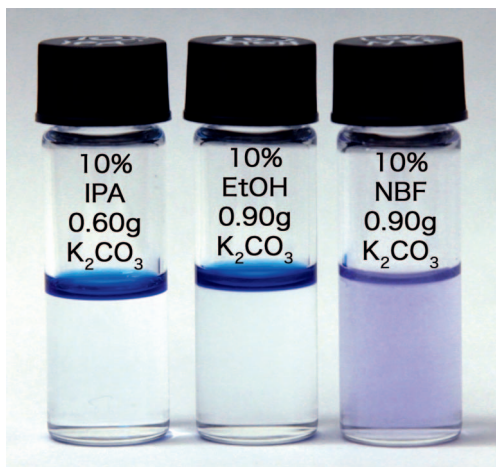
Figure 2. Photograph of salting-out tests (with one drop bromothymol blue indicator in 2 ml of fluid) (left to right): 10% IPA with Test A (0.60 g K_2CO_3 ); 10% EtOH and 10% NBF with Test C (0.90 g K_2CO_3 ) (© I. Finkelde).
