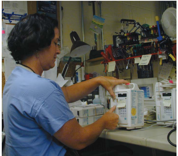
Technician T.C. Bugbee performs functional tests on infusion pumps at Fletcher Allen Health Care in Burlington, VT.
