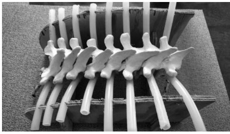
Figure 1 - Photograph of the model constructed of plastic thoracic vertebrae T2-T9 and a rib structure of polyethylene tubing supported in a plywood carriage.
