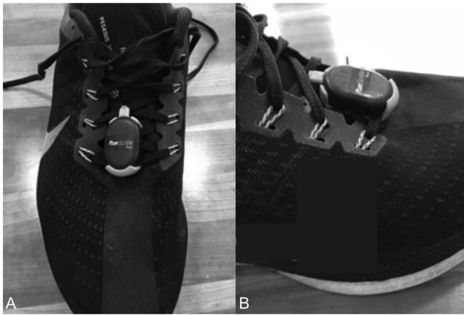
Figure 1. Illustration of the position of an inertial measurement unit sensor on a running shoe.
