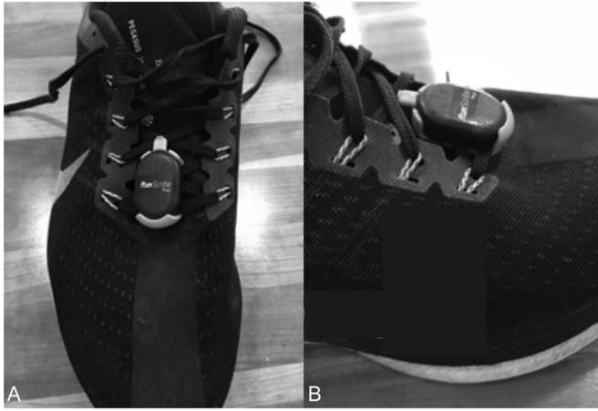
**Figure 1.** Illustration of the position of an inertial measurement unit sensor on a running shoe.
