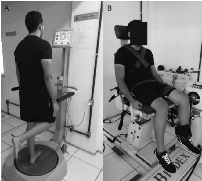
Figure 1. Biodex System 4 Pro (Biodex Medical Systems Inc, Shirley, NY). A, Postural-stability test. B, Isokinetic test for knee extension and flexion.
