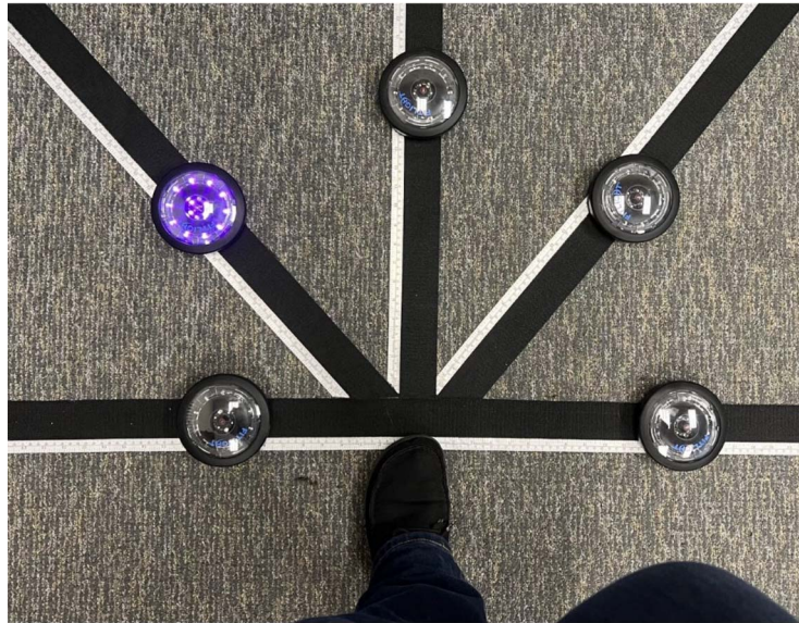
Figure 1. The lower extremity visuomotor reaction time task. The active limb is the right, and the stable limb is the left. Shank length was used to place lights. The light lateral to the limb being tested was placed at half-shank length.
