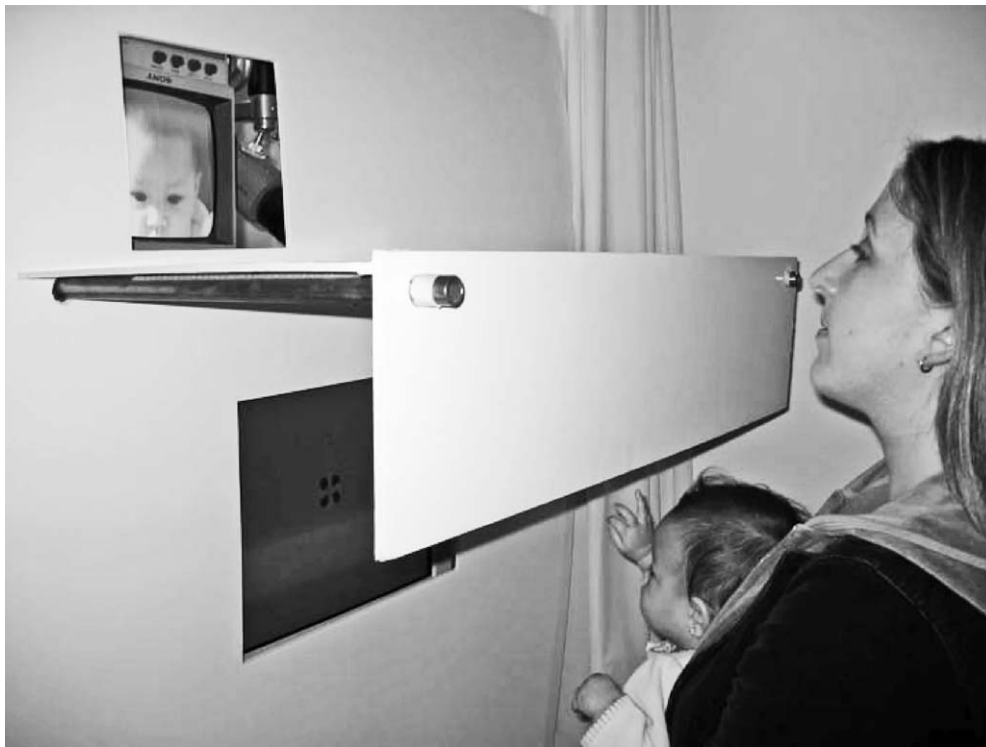
Figure 4. Forced-choice preferential looking (FPL) technique used in the current study. On each trial, an upright and inverted stimulus appeared on the left and right side of the monitor, respectively, and an experimenter used the subject's head turning and eye gaze behavior (viewed with a video camera aimed at the infant's face, projected onto the camera monitor above) to judge which side the subject preferred. (In this example, an infant is being tested. However, adults were also tested using FPL.) Note that the experimenter was blind to the stimulus locations because a piece of cardboard blocked her view of the video monitor. Above chance (i.e., > 50% correct) scores indicate a preference for the upright over the inverted stimulus.
