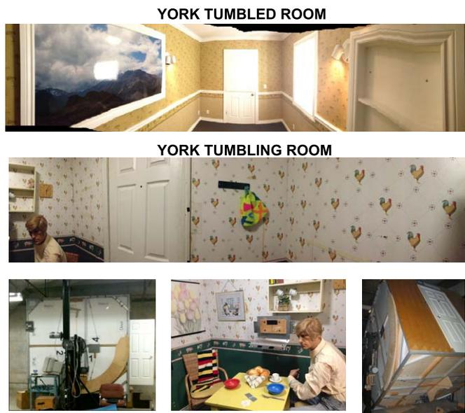
Figure 1. Photographs of the York Tumbled (top) and Tumbling (bottom) facilities. The Tumbled Room measured 244 cm  $\times$  244 cm  $\times$  366 cm (8 ft  $\times$  8 ft  $\times$  12 ft) and the Tumbling Room is 244 cm  $\times$  244 cm  $\times$  244 cm (8 ft  $\times$  8 ft  $\times$  8 ft). The panoramic views of each room were taken with the photographer on his back relative to gravity (photographs by the author, LRH).
