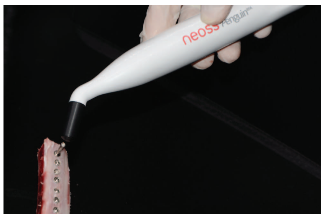
FIGURE 2. The probe of the Penguin RFA was held 1 mm from the multipeg at a 90° angle and the implant stability quotient was registered on the digital screen of the instrument for each implant.
