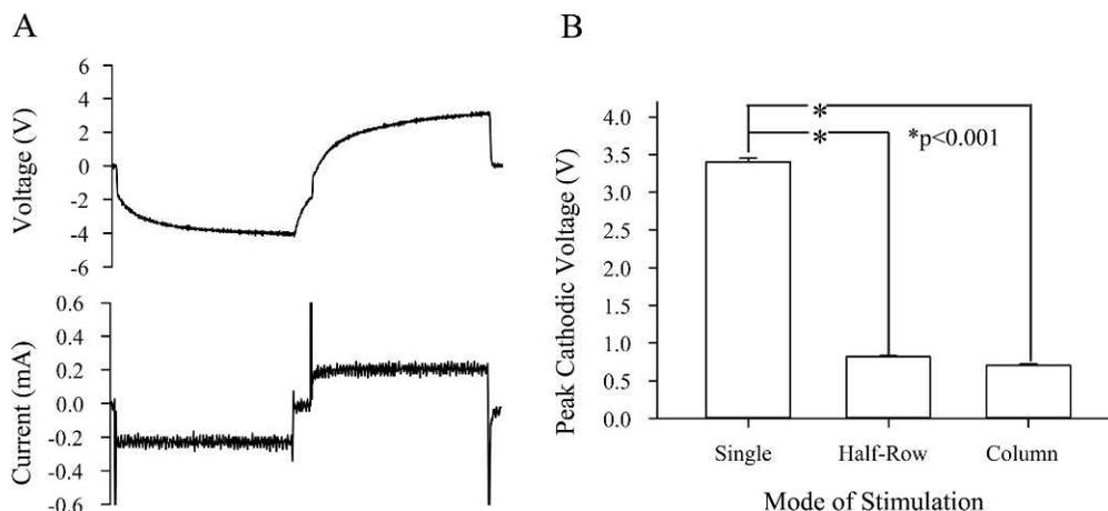
**FIGURE 2.** (A) Typical voltage and current waveform recorded in vivo from stimulation of a single electrode on the suprachoroidal array (200  $\mu$ A, 250  $\mu$ s). (B) Peak cathodic voltages measured with single electrodes, half-rows, and columns from all experiments. Voltage excursions measured for lines were found to be significantly lower than those measured for single electrodes.
