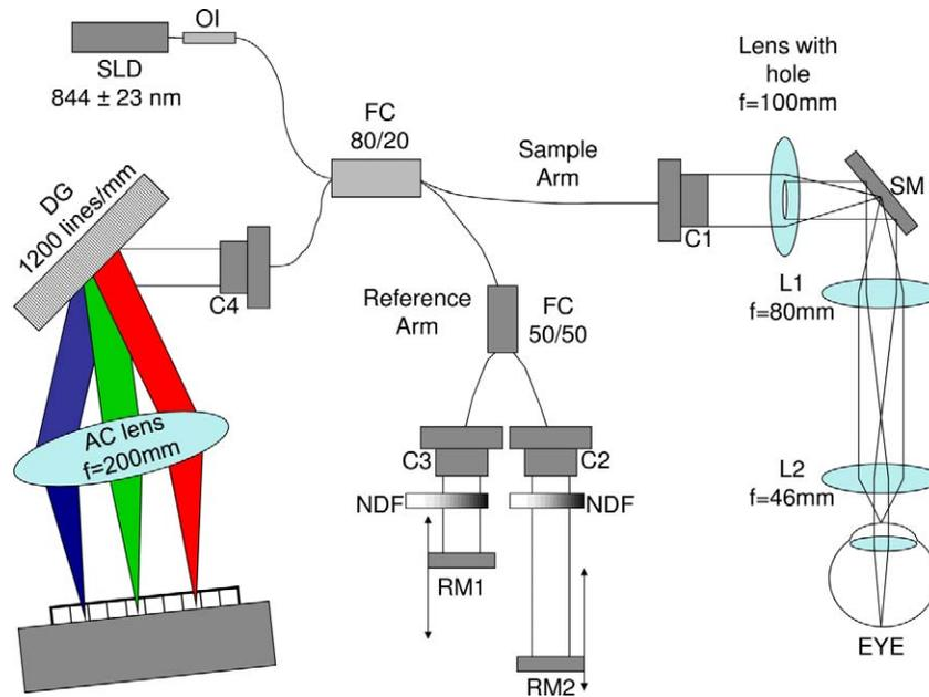
**FIGURE 1.** Layout of the optical system. Different components are the superluminescent diode (SLD), optical isolator (OI), fiber coupler (FC), collimator (C1-C4), lens (L1-L2) with focal length ( $f$ ), scanning mirror (SM), reference mirror (RM1-RM2), neutral density filter (NDF), dispersion grating (DG), and achromatic (AC) lens.
